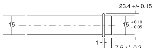
Fig. 9. Pipe end for "O"-ring connection
